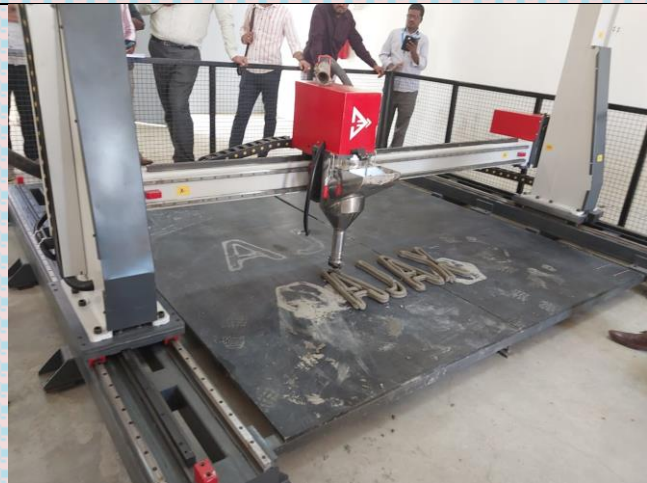
Demonstration of 3D Concrete Printing Equipment
